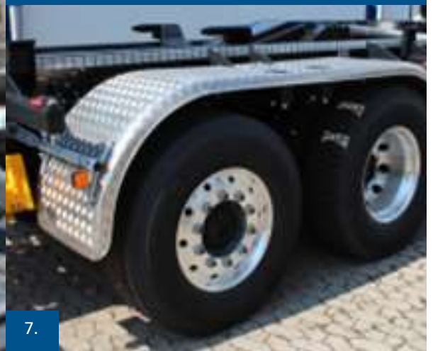
7. Mudguard in aluminium ribbed design.
